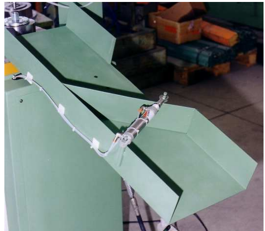
Chute to exit pieces
