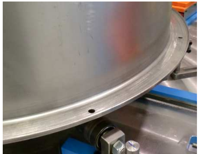
Flanged and punched ferrule Ø900 mm
